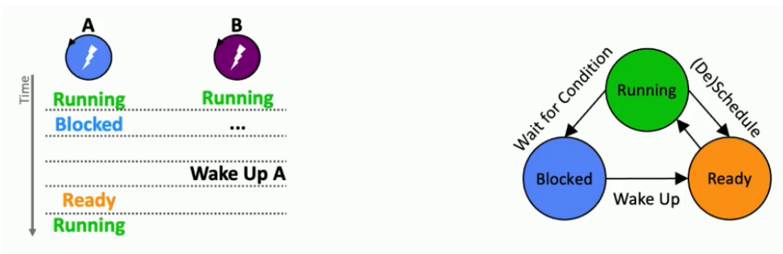
Figure 77: Note that the only way a thread can be blocked is if it is waiting for a condition to happen. If that condition happened and a signal arrives at the thread, then it “wakes up.” Condition variables allow these thread to go in and out of the blocked state.
