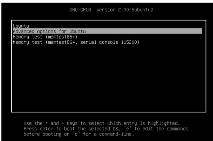
Figure 11: GRUB menu on my screen. Ubuntu does not display the GRUB menu by default. To see GRUB during boot you need to press the right-hand SHIFT key during boot.
