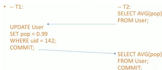
Figure 54: In T2, we first compute an average of say 0.6. Then in T1 we update the popularity and commit. Then in T2, we take the average again, getting 0.8, and finally commit. T2 ends up reading two different states of the database.
