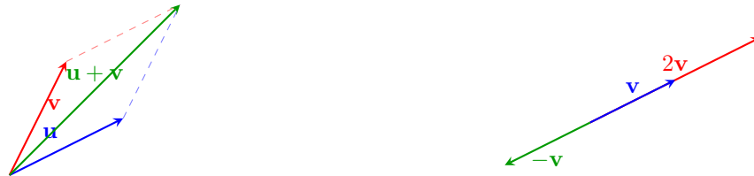
(a) Addition is visualized using the “parallelogram rule.” (b) Scalar multiplication is simply a stretch of the vector.
