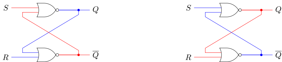
(a) If we send a signal R = 1 , then Q = 0 , and even if we reset R = 0 , Q is still locked at 0. (b) If we send a signal S = 1 , then Q = 1 , and even if reset S = 0 , Q is still locked at 1.
