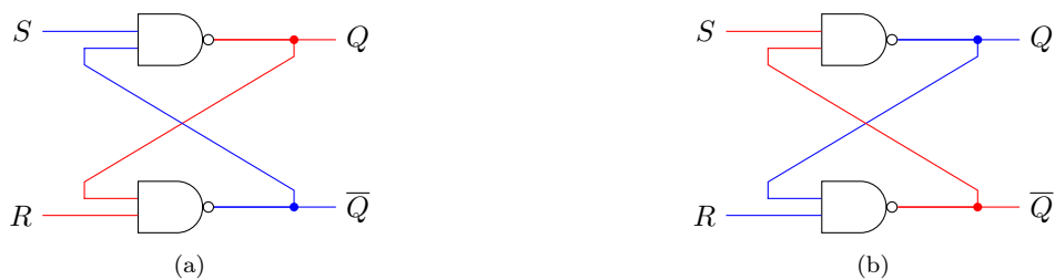
Figure 7: If we send a signal S = 0 , then Q = 0 , and even if reset S = 1 , Q is still locked at 0.
