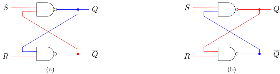
Figure 6: The default state is R = 1, S = 1 , i.e. they are both high states , and Q may be either 0 or 1. This is known as an active low SR latch .
