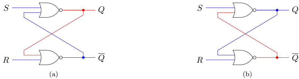
Figure 3: Two possible initial states. The default state is R = 0, S = 0 , which are both low states , and Q may be either 0 or 1.
